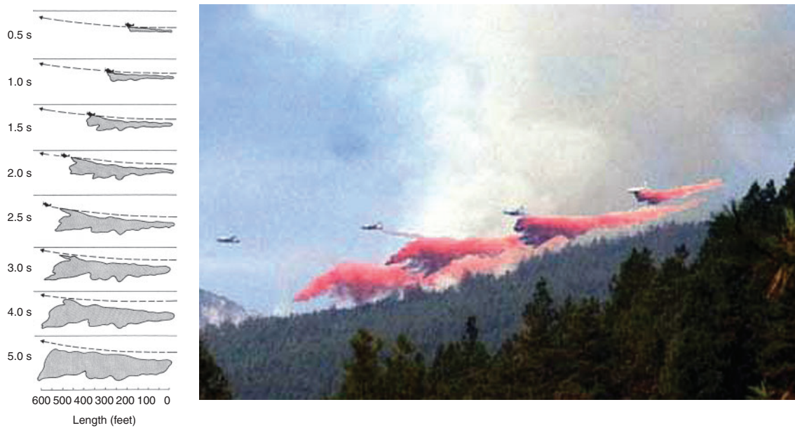
Fig. 1. Schematic representation (George and Blakely 1973) and sequence of images of a retardant aerial drop (Blodgett Fire (US), August 2000). (Scale: 1 foot = 0.30 m.) (Photo credit: Bruce Weide (Wild Sentry, Hamilton, MT).)
