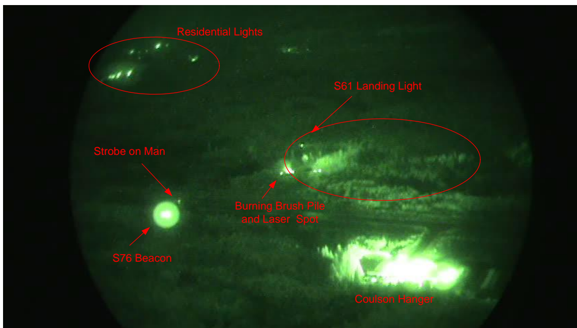
Figure 16. NVG view of other aircraft during the operation. Movement of the aircraft and the flashing beacons made identification unmistakable.
