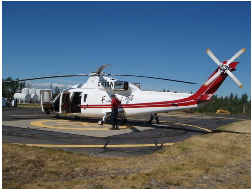
Figure 4. S-76 Firewatch helicopter with infrared camera and gyro stabilized ball under the aircraft nose.
