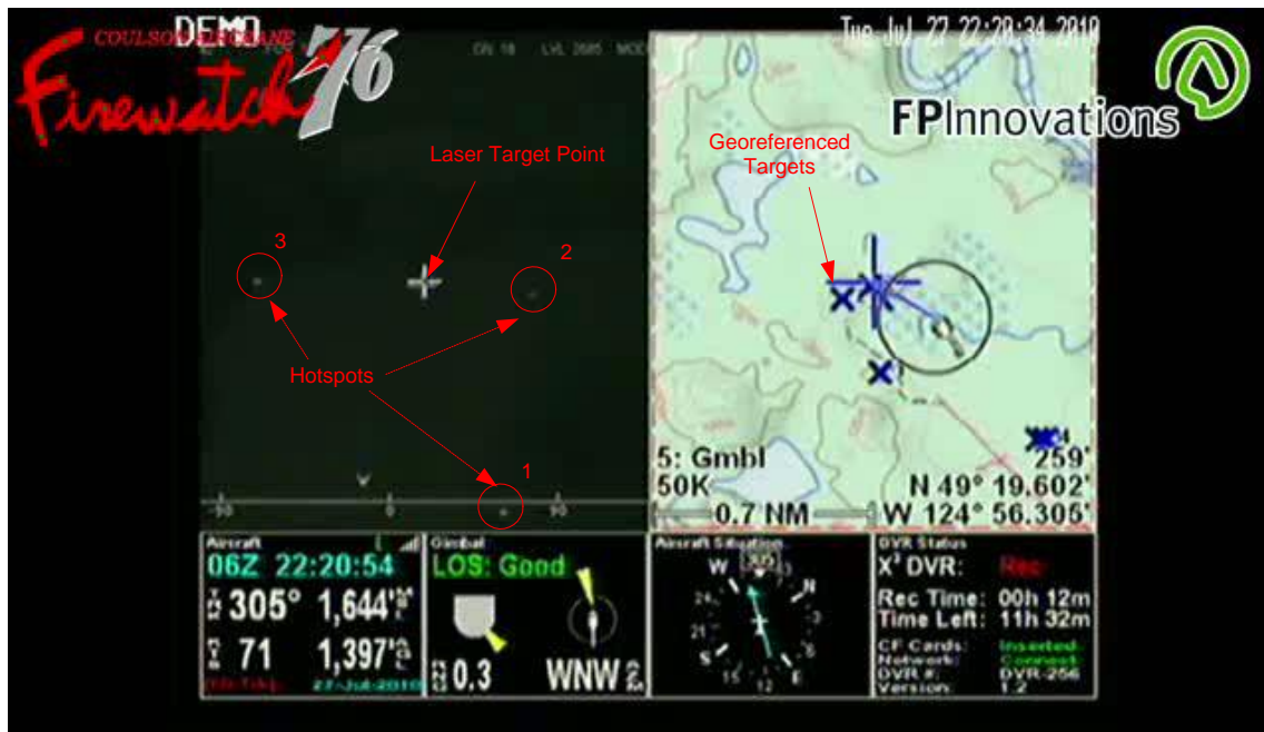
Figure 5. Screen shot from the S76 showing IR screen and map screen for targeting and recording hotspots.
