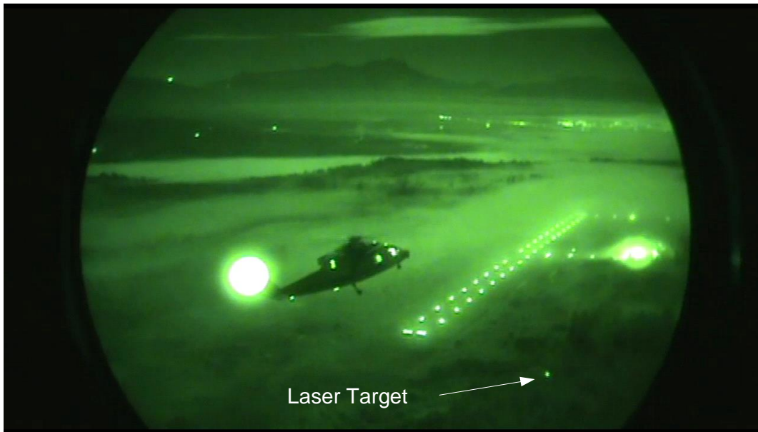
Figure 6. NVG view of the S-76 and IR laser target designator illuminating the ground.
