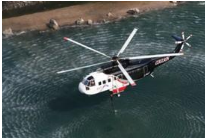
Figure 2. Coulson S-61 with 4000 litre belly tank and snorkel.
