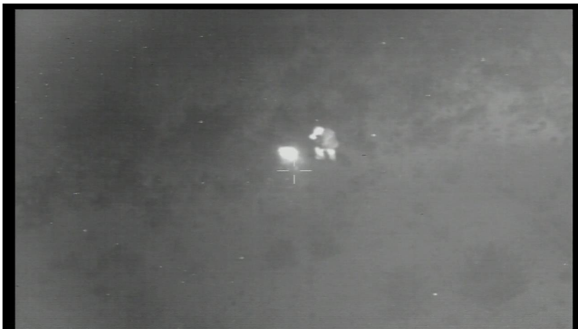
Figure 15. IR image of man and hotspot. Image from 2000 feet AGL, zoomed in. Note reflective stripe on shirt is barely visible.
