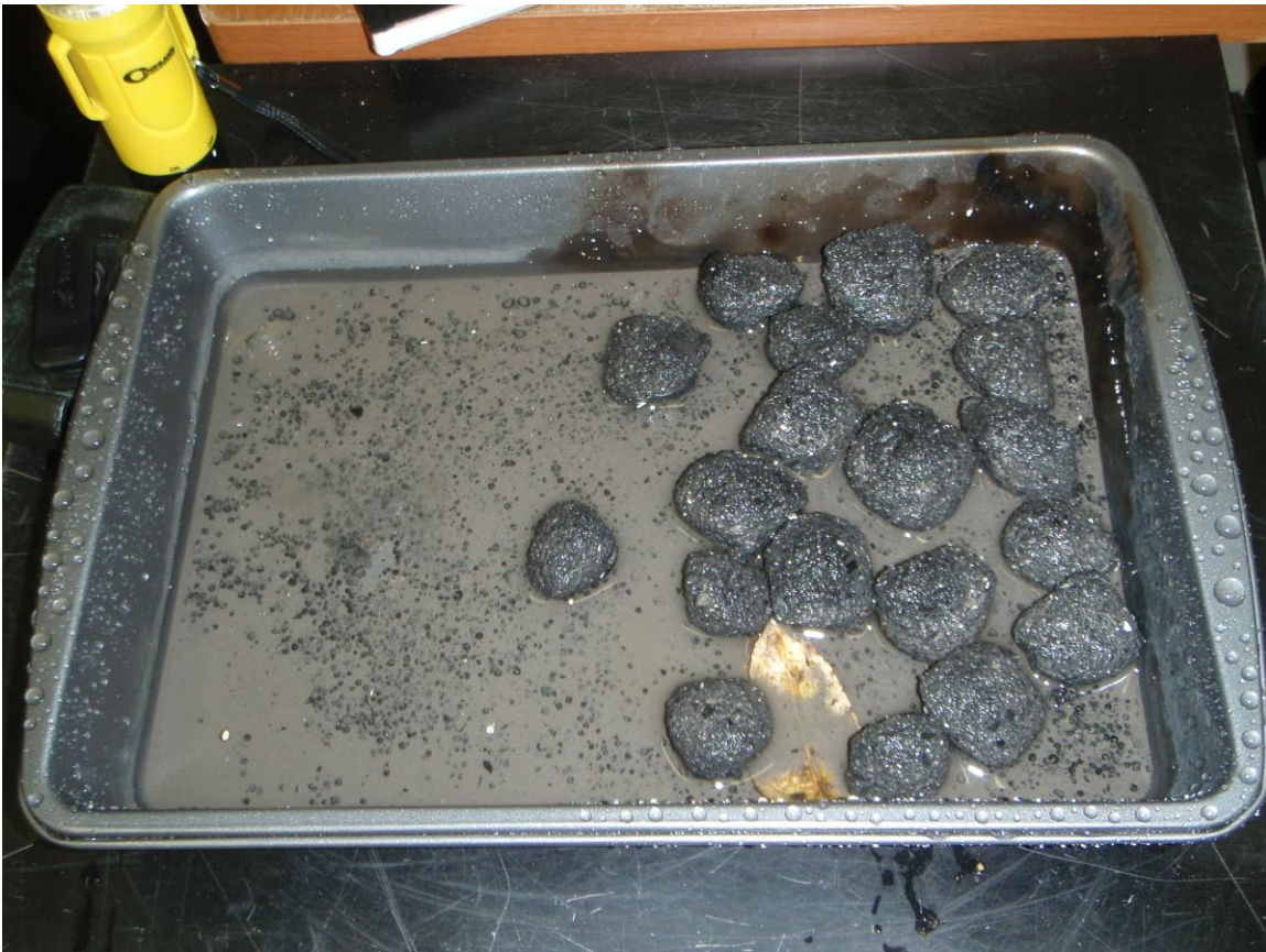
Figure 13. Water accumulated in hotspot target pan after two drops from the S-61 during night operations.
