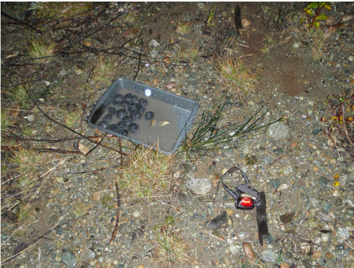
Figure 11. Target after the first drop and flashing beacon for aiding water delivery. The flash was clearly visible in the S-61 under NVG. Note the amount of water in the pan was enough to extinguish the briquettes.
